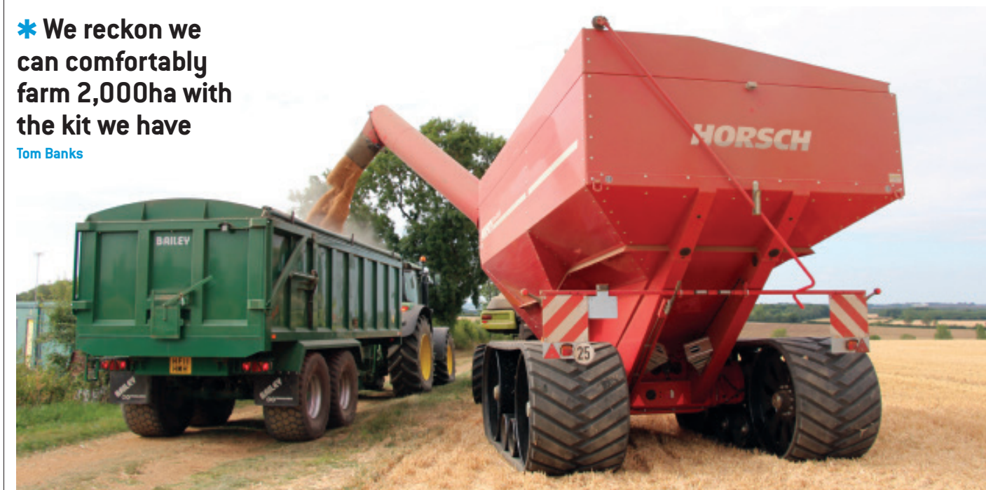
Courteenhall Farms' giant Horsch chaser bin can hold 28t of wheat. The 60cm-diameter auger (shown here folded) discharges its load in a barn-busting 90 seconds.
