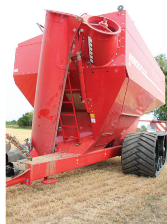
Courteenhall Farms' giant Horsch chaser bin can hold 28t of wheat. The 60cm-diameter auger (shown here folded) discharges its load in a barn-busting 90 seconds.
