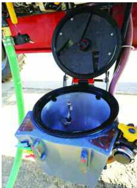
*The swivelling induction bowl is well positioned – not too low for liquid filling, but not too high to put in powder.*
