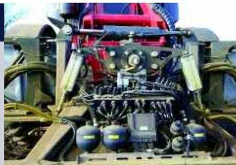
*The boom box, at the heart of BoomControl Pro, determines sprayer nozzle choice and maintains the boom height.*
