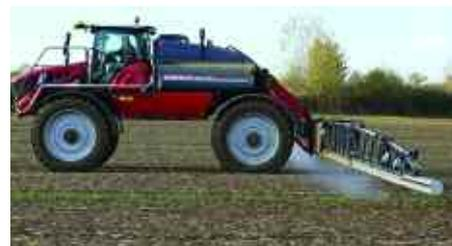
*Horsch's patented boom technology separates the boom from the machine so it works independently from how the machine is travelling across the field.*
