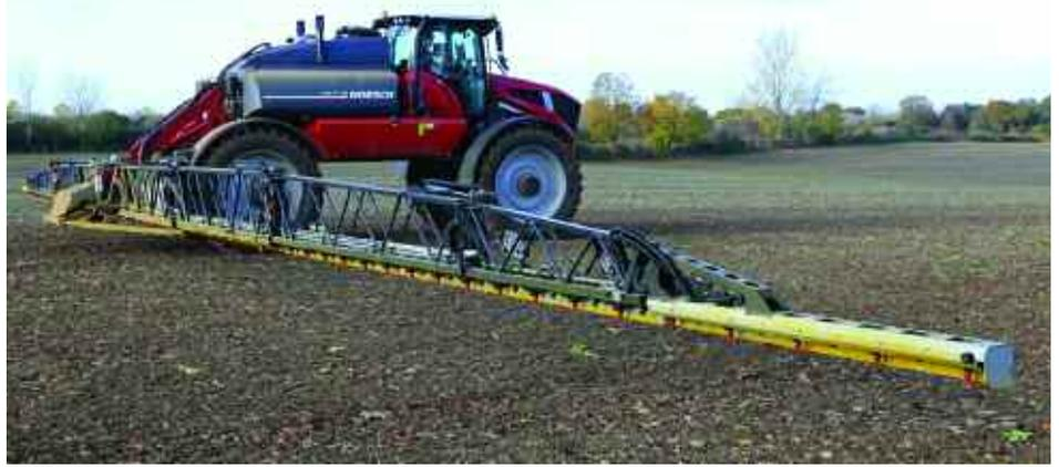
Courteenhall's CTF system is based on 12m passes, with the sprayer operating at 36m passes using the same tramlines.
