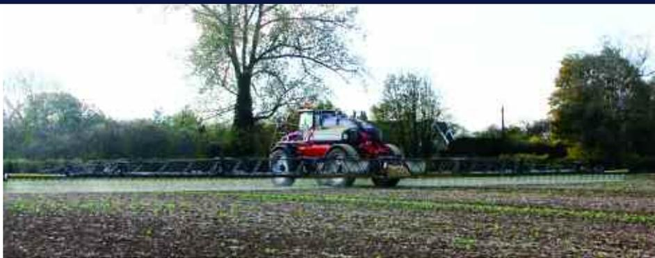
Nozzles at 25 cm spacings in combination with boom control allows a boom working height of 30cm which means a large reduction in drift.
