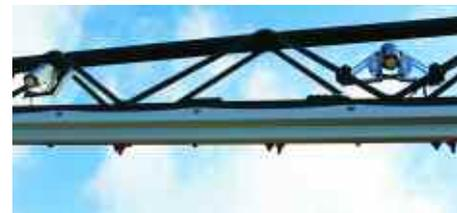
Sensors mounted on the boom allow the machine to adapt to changes in terrain and maintain the lowest possible working height.
